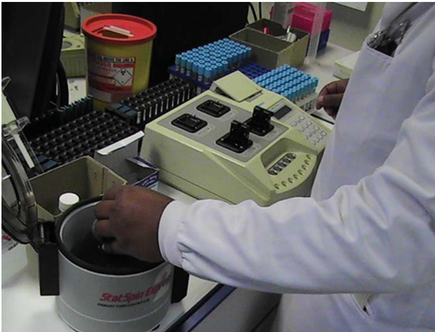
Microcentrifugation using the StatSpin Express 2 can reduce centrifugation time without compromising the quality of results for routine coagulation tests.
