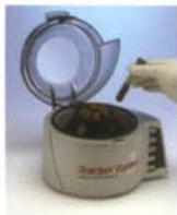
The StatSpin Express 3 Primary Tube Centrifuge holds eight tubes up to 10 mL.
